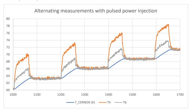
As the thermal diffusivity of copper is very high, steady-state conditions can be reached very quickly during both the calibration and conductivity measurement phases.
