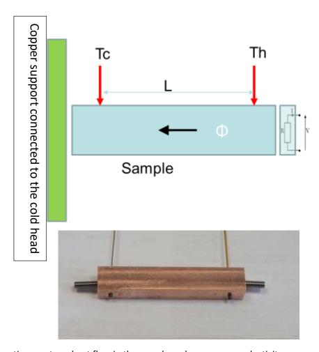
Pulsed heating creates a heat flow in the sample and measures conductivity:
