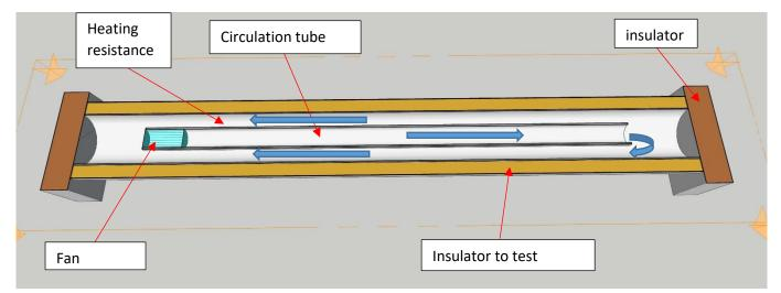
In the diagram the blue arrows represent the convection air flow. Centering guides keep the circulation tube central. A fan is placed inside the circulation tube. Thermocouples are fixed on each tube in order to check the homogeneity of the temperature in the central tube.
